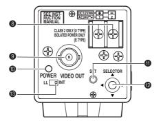
[DC 12V, AC 24V] Power input terminals To input DC 12V or AC 24V power.
